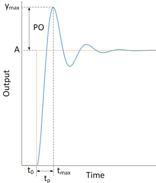
*Response of a second-order system to a step input*
