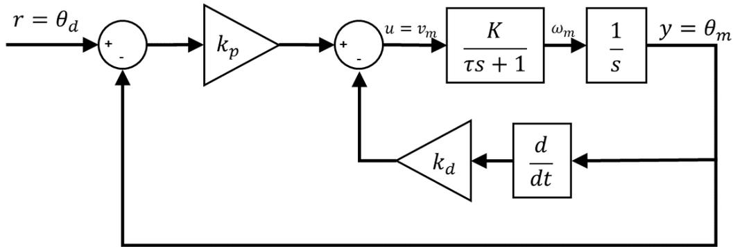
*Block diagram of rate feedback control*
