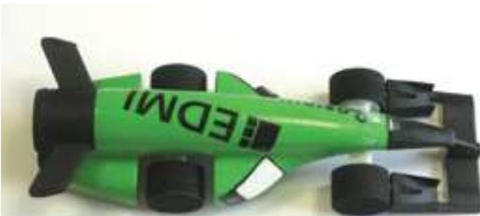
As part of the F1 in Schools Challenge, 3D Printers are ideal for printing front & rear wings, wheels, wheel support systems and nose cones – allowing teams to enhance and fine-tune their car designs.
