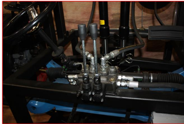
Pneumatic Controls to Simulate Various Road Conditions
