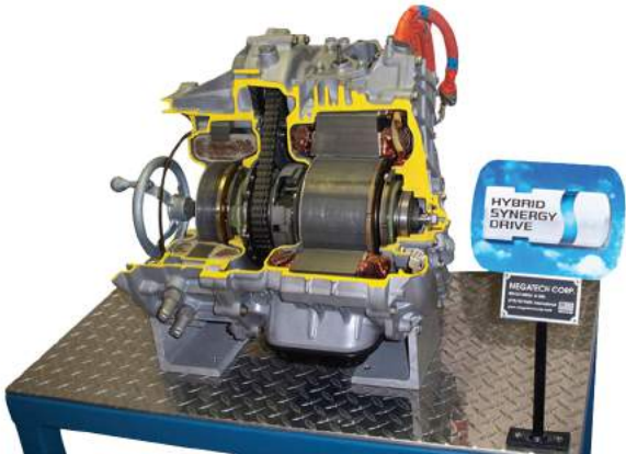
MEGART34500 Hybrid Engine / Generator Cutaway
