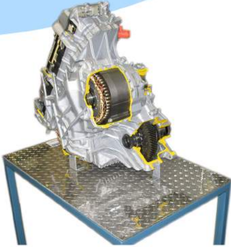
MEGART34500 Hybrid Engine / Generator Cutaway
